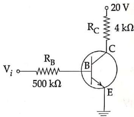
In the circuit shown in the figure, the input voltage  $V_i$  is 20 V,  $V_{BE} = 0 \text{ V}$  and  $V_{CE} = 0 \text{ V}$ , what are the values of  $I_B$ ,  $I_C$  and  $\beta$  ?
