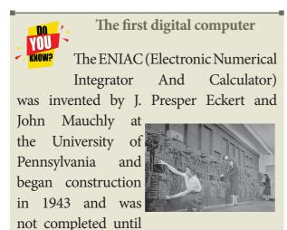
1946. It occupied about 1,800 square feet and used about 18,000 vacuum tubes, weighing almost 50 tons. ENIAC was the first digital computer because it was fully functional.
