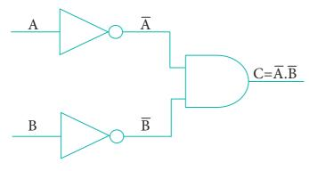
Fig. 2.9 Logic circuit of Bubbled AND Gate
