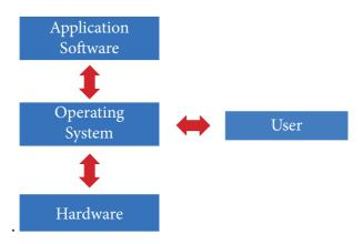
Figure: 4.2 Interaction of Operating system and user
