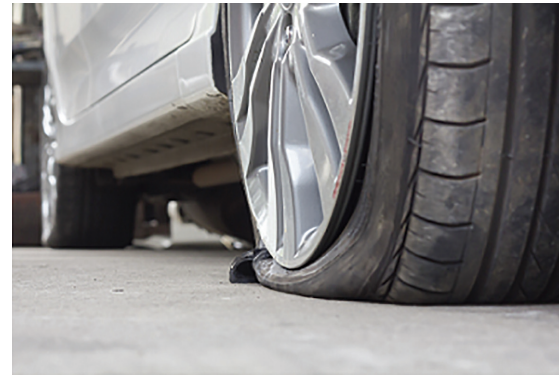
Figure 8.29 (a) When the tyre bursts the air expands so quickly that there is no time to exchange heat with the surroundings.
