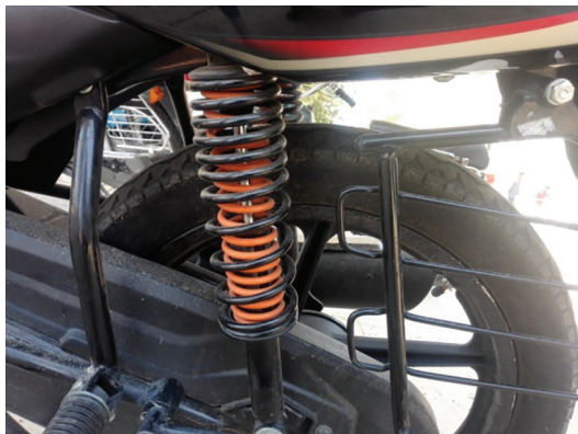
Figure 10.16 Combination of spring as a shock-absorber in the motor cycle
