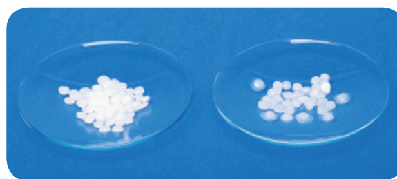
Figure 9.11 Deliquescence in Sodium hydroxide
