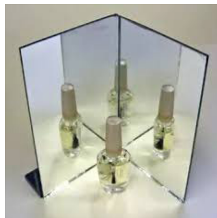
Figure 6.5 Images formed by inclined mirrors
