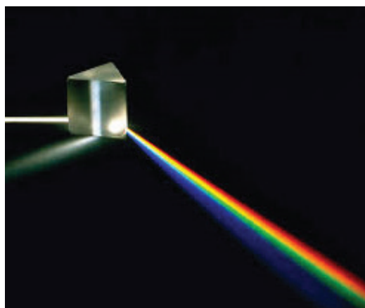
Figure 5.12 White light passed through prism – dispersion
