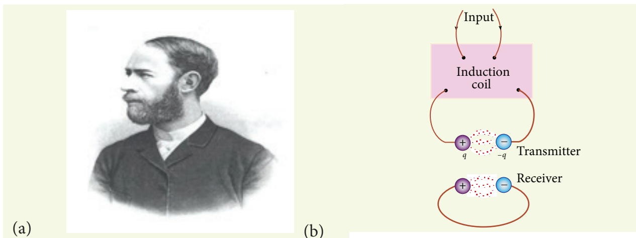
Figure 5.7 (a) Heinrich Rudolf Hertz (b) Schematic diagram of Hertz apparatus
