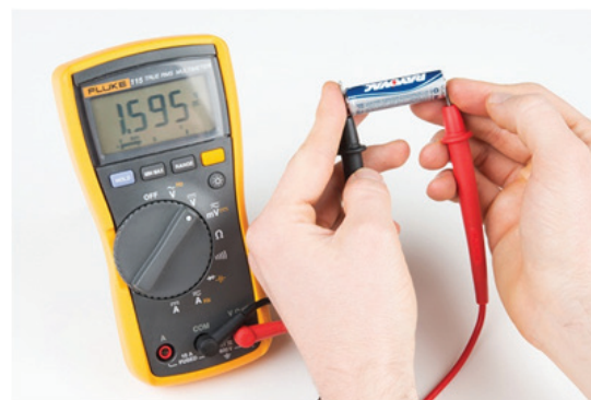
Figure 2.19 Measuring the emf of a cell
